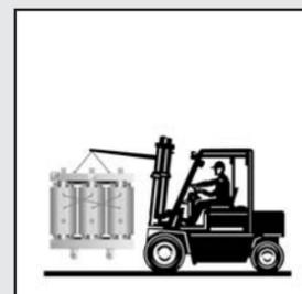
Fig. 10 Handling by means of a forklift
