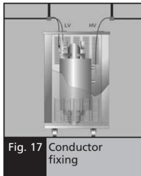
Fig. 17 Conductor fixing
