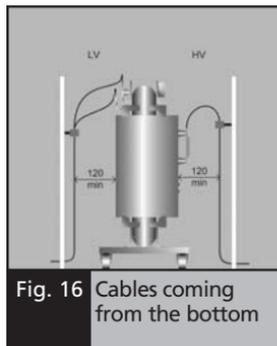
Fig. 16 Cables coming from the bottom
