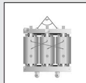
Fig. 9 Handling by means of any overhead-travelling crane
