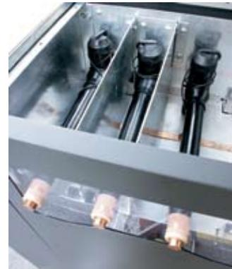
The **switch compartment**, which is sealed for life, houses the switching and breaking switchgear, with SF<sub>6</sub> gas as the insulating medium. Built of stainless steel, it has been designed and tested to withstand an internal arc up to 25 kA/1 s. The gases generated as a consequence of an internal arc are cooled and can be channelled through a relief duct located at the back.
